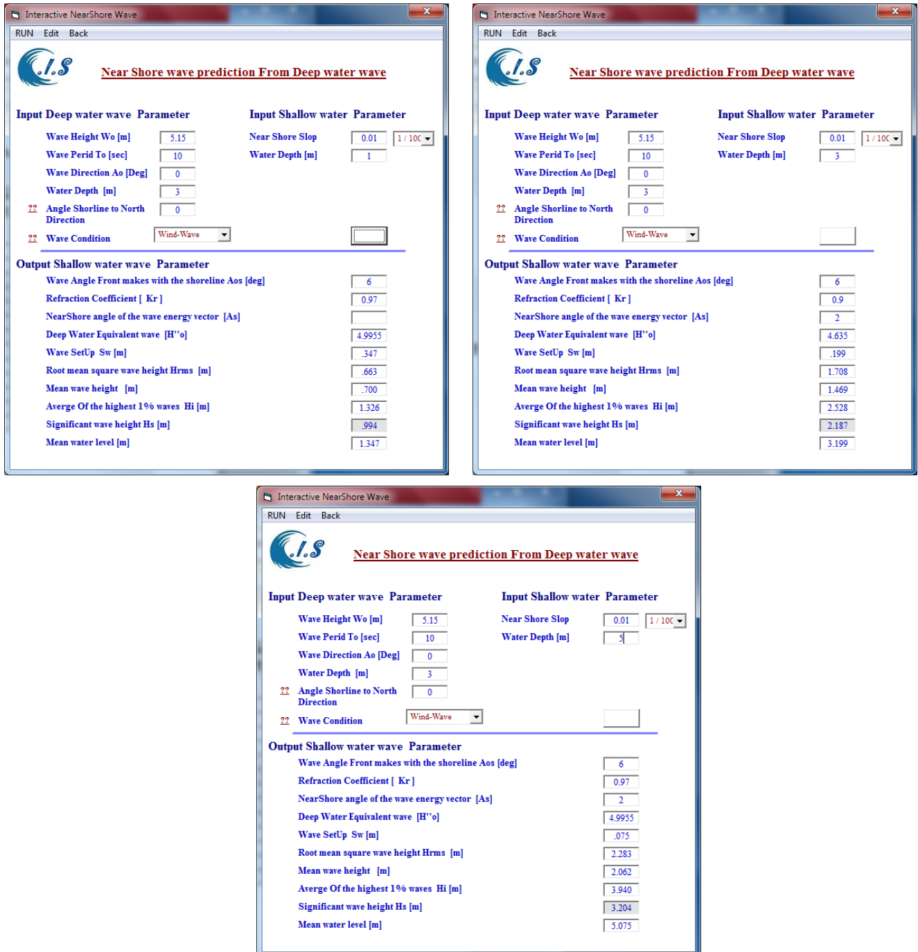
Figure 6. NShore model interactive option page with [ H_0 :5.15m T_0 :10sec A_0 :0° at water depth d = 1,3,and 5] beach slop [ 1/100]
