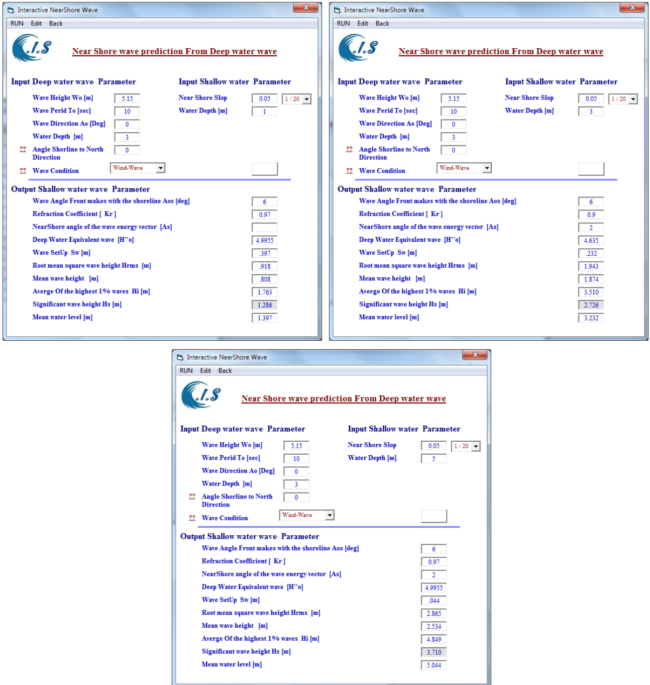
Figure 8. NShore model interactive option page with [ H_0 :5.15m T_0 :10sec A_0 :0° at water depth d= 1,3, and 5] beach slop [ 1/20]
