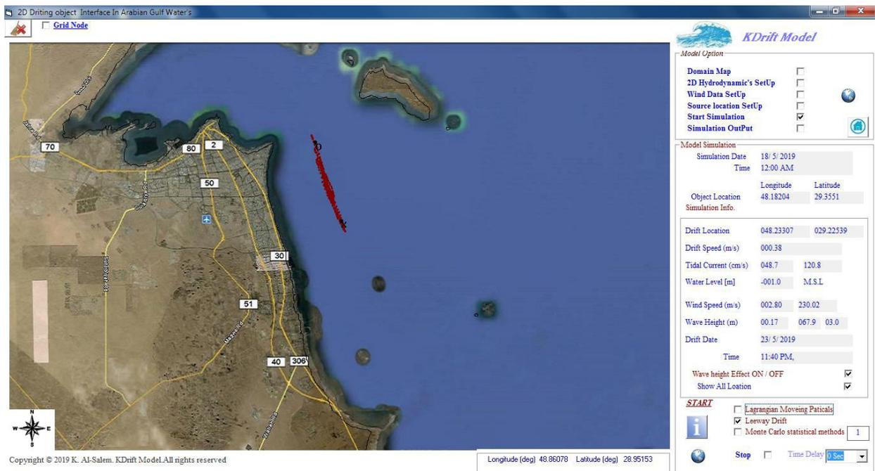
Figure 10. Drift Object Simulation by Leeway Drift Method
