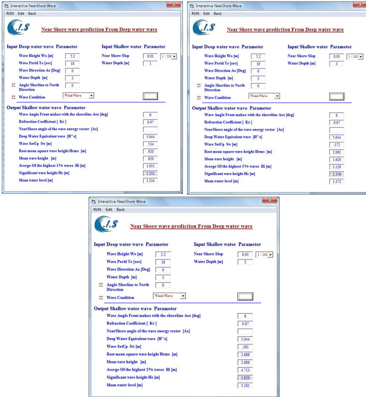
Figure 13. NShore model interactive option page with [ $H_0:5.2$  m  $T_0:18$  sec  $A_0:0^\circ$  at water depth  $d= 1,3,$ and  $5$ ] beach slop [  $1/100$ ]  $H'_0: 5$ m
