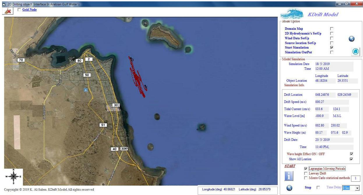
Figure 8. Drift Object Simulation by Lagrangian Moving Particles theory
